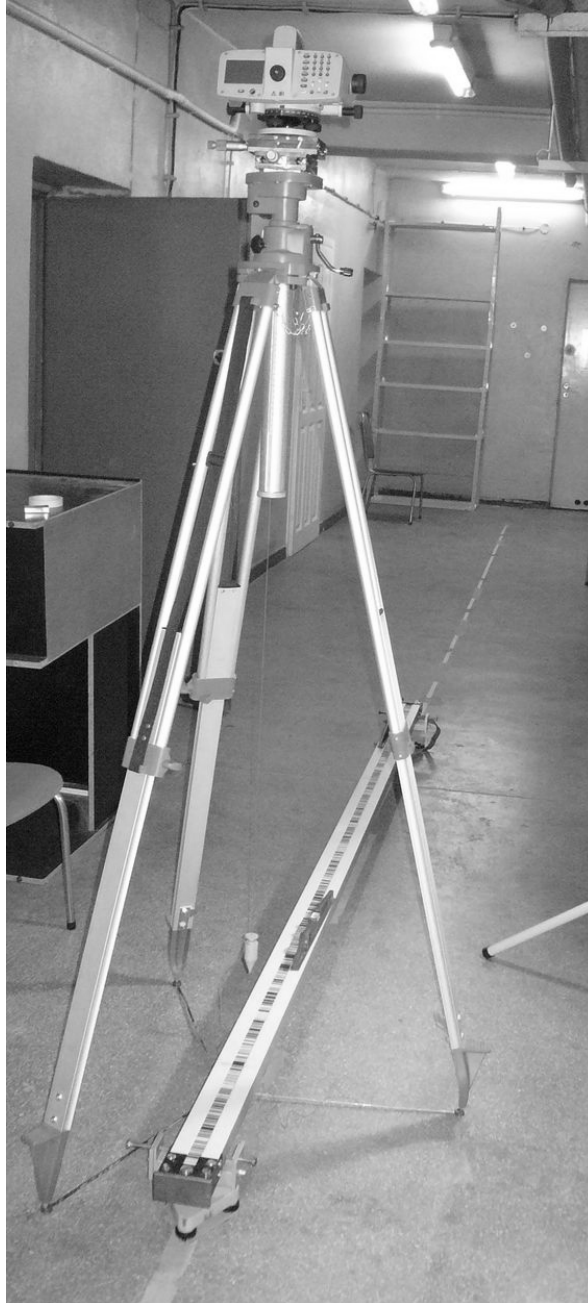
Fig. 2. View of a leveling batten initially set along the measured segment and leveled by a plumb-line.
