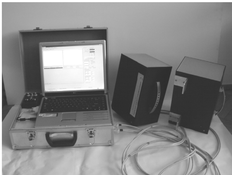
Fig. 1. The device for measuring verticality and straightness of the shaft guides.
