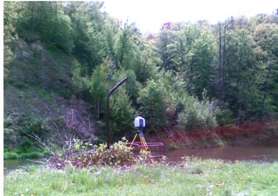
Figure 5. Scanner at the river Nysa Klodzka, in front of landslide forehead.
