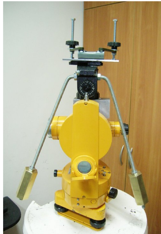
Fig. 3. A setting pipe level.
