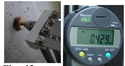
Fig. 13. – measurement of tension and pressure zones.
