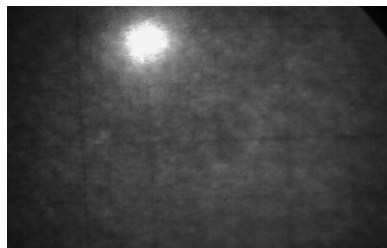
Fig. 9. Picture of a registered fleck for measurement receiver movement of +8 mm from initial setting.
