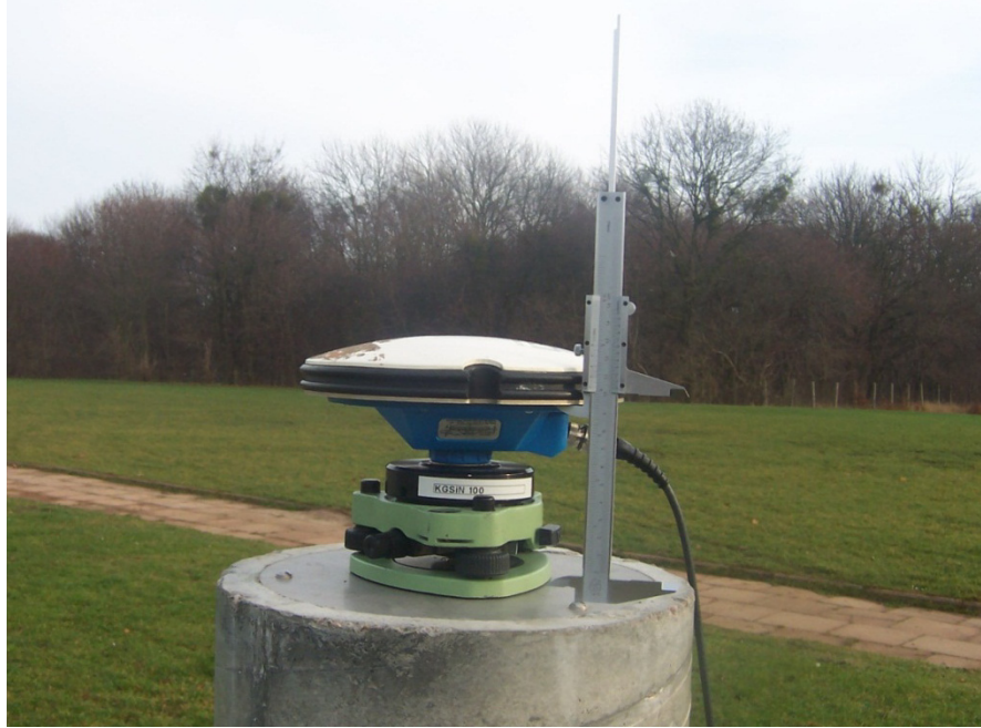
Fig. 3. Antenna height measurement over one of the three benchmarks at the reference point.
