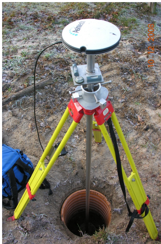
Fig. 4. Collecting GPS observations at a monitored point with use of the patented pole (UWM nr 90-402/45/2007).
