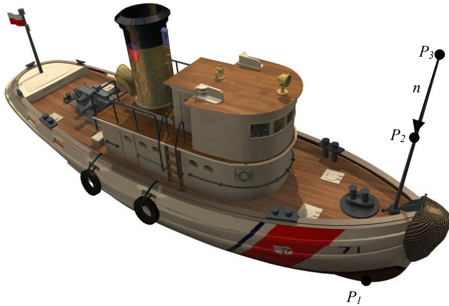
Fig. 2. Location of antennas and transducer with three colinear points method.
