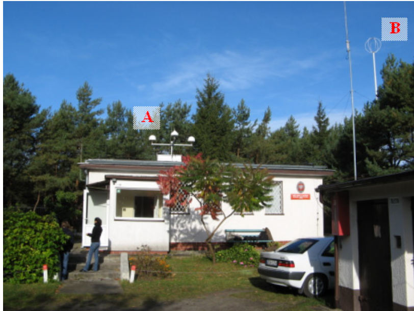
Fig. 2. View of nautical station in Dziwnow; (A) GPS antennas, (B) transmitting antenna.
