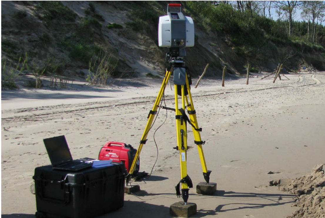
Fig. 4. Leica ScanStation 2 scanner used in the survey.
