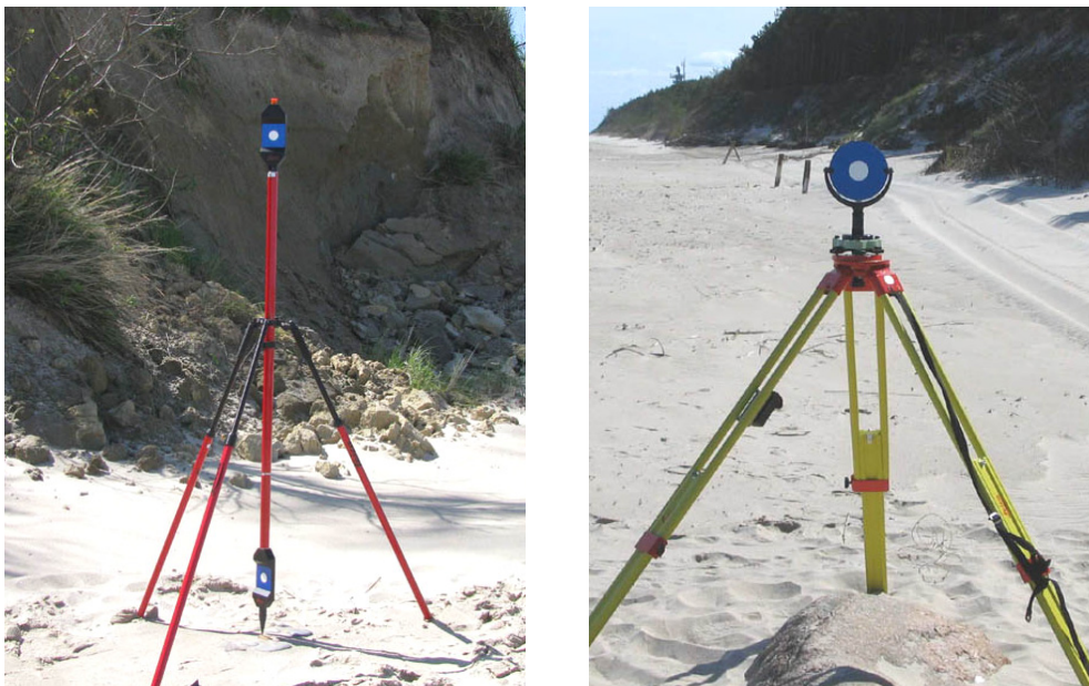
Fig. 6. Example of common points signalization for different point clouds.
