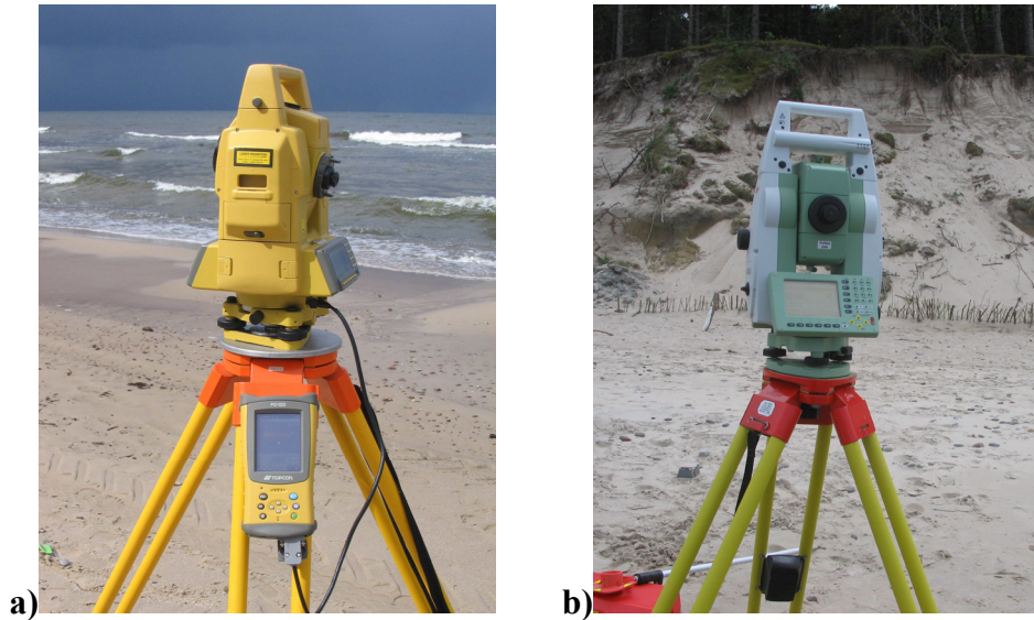
Fig. 2. Tacheometers used in the survey: a)Topcon GPT-8203A SCAN, b)Leica TPS1200.
