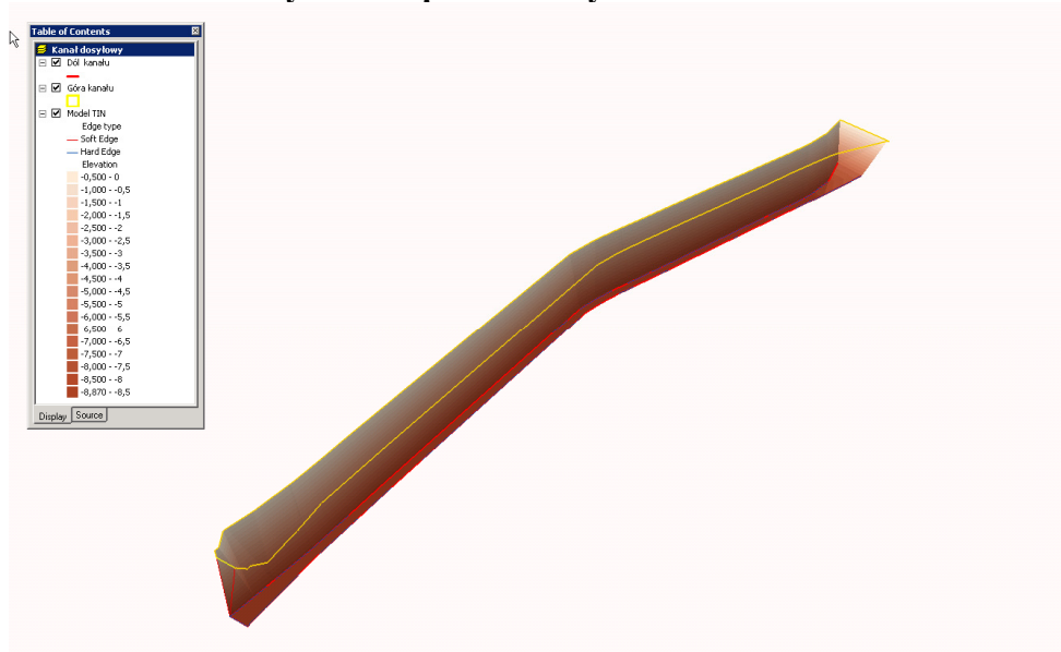
Fig. 9. Spatial model of the channel – TIN, interpolated on the basis of the archival materials and technical documentation made available.
