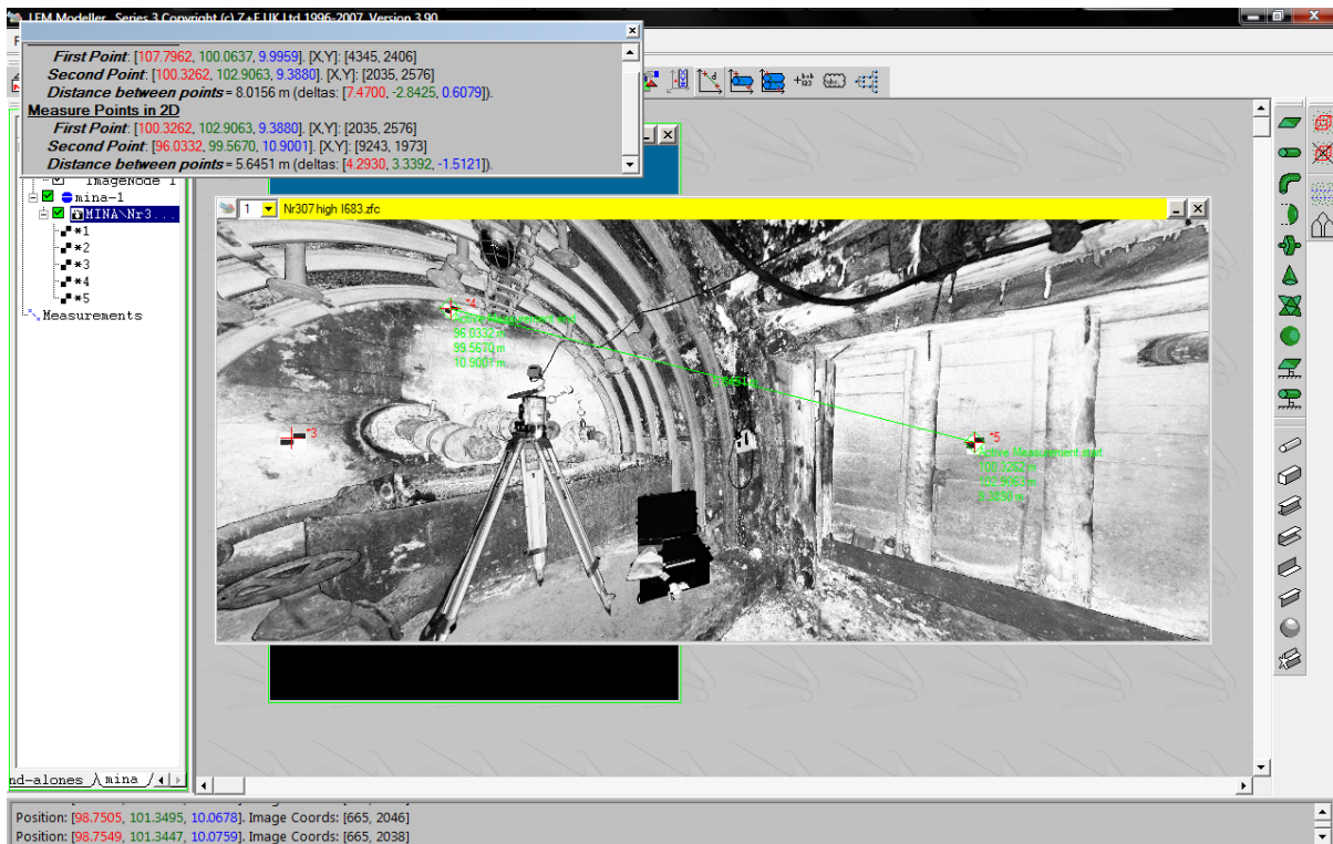
Fig. 7. Finding the distance and coordinate increments between control points in the cross-cut- measurements on the basis of “intensity” images (LFM Modeller).
