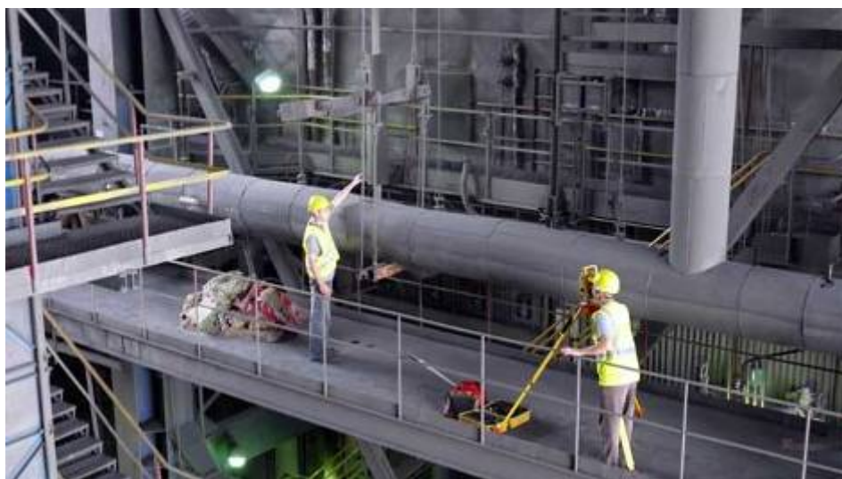
Fig. 1. Geodetic measurements in CHP power station.
