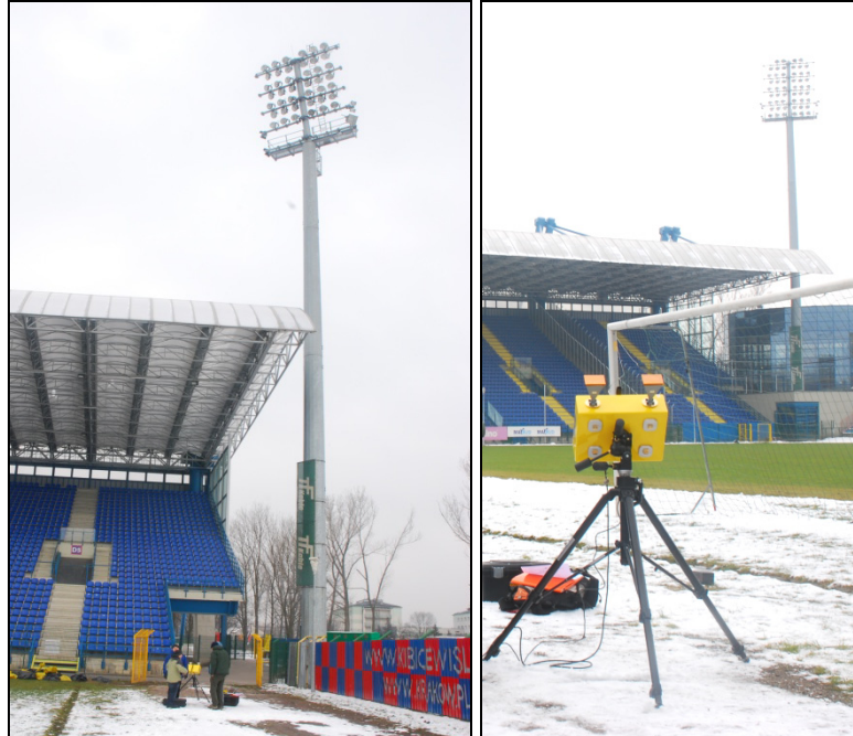
Fig. 2. IBIS-S during field test at the H. Reyman municipal stadium in Cracow.
