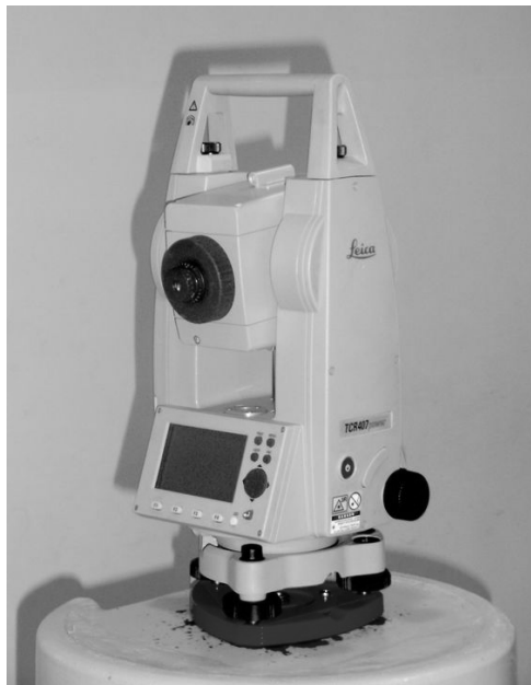
Fig. 3. Electronic tachometer Leica TCR407 power on an observation post.
