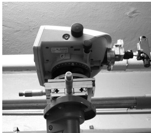
Photo 3. View of the instrument with connected pentagonal prism
