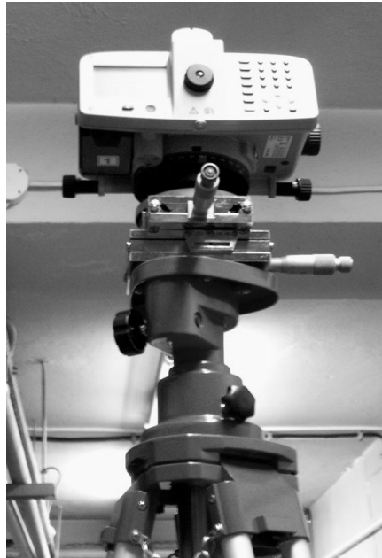
Photo 4. View of instrument placed on micrometric stage
