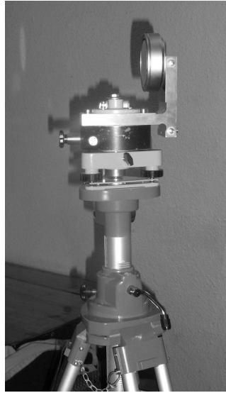
Photo 6. Reflection device in the process of breaking the level aiming line
