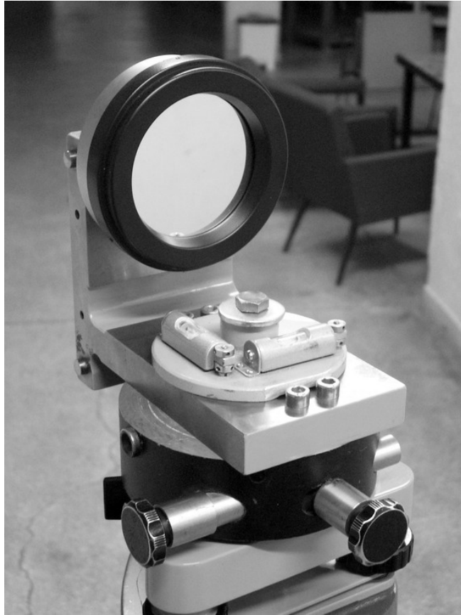
Photo 3. Reflecting device on measuring post
