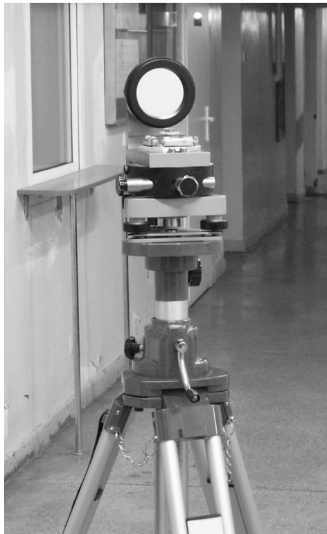
Photo 4. The reflecting device is placed on a tripod where a measuring head is situated in the vertical position
