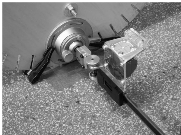
Fig. 5. View of a prototype of the device while in use, concerning a controlled point on the rim of a wheel.
