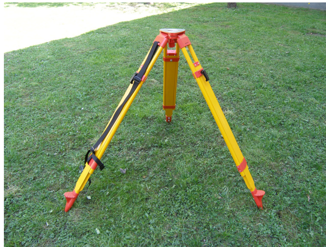
Fig. 2. A traditional tripod with extensible legs.
