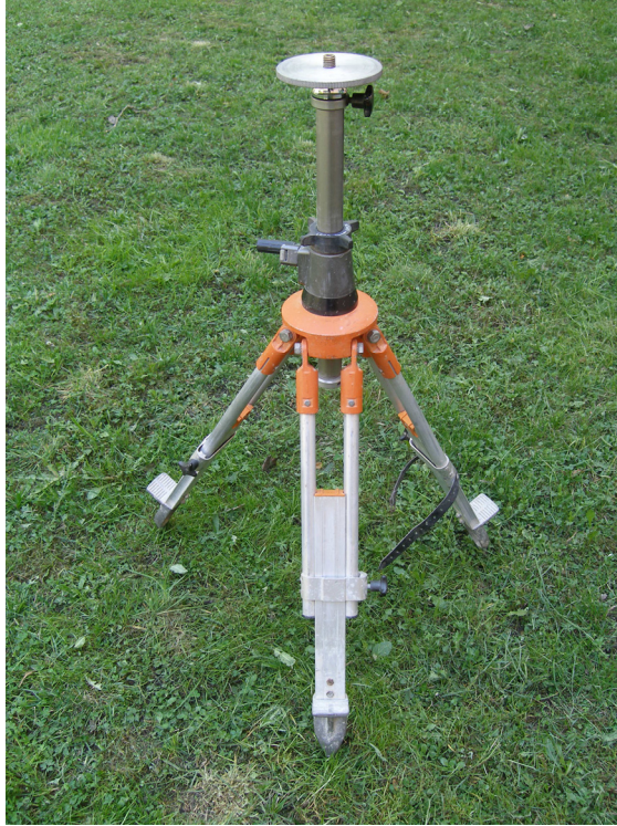
Fig. 3. A tripod with a vertically adjustable head.
