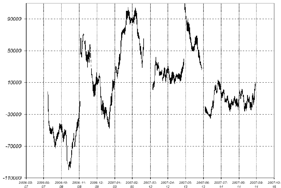
Fig. 13. Graph of gravity changes [ \text{nm/s}^2 ] as observed at the Józefosław Observatory using a D-196 gravimeter.
