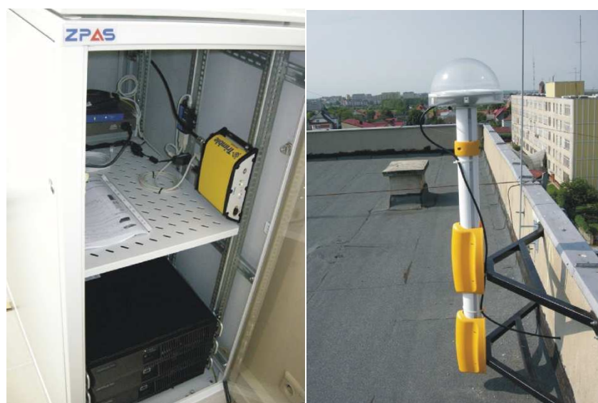
Fig. 1a. ASG-EUPOS LOMZ station as an example of a GPS station established during the project.
