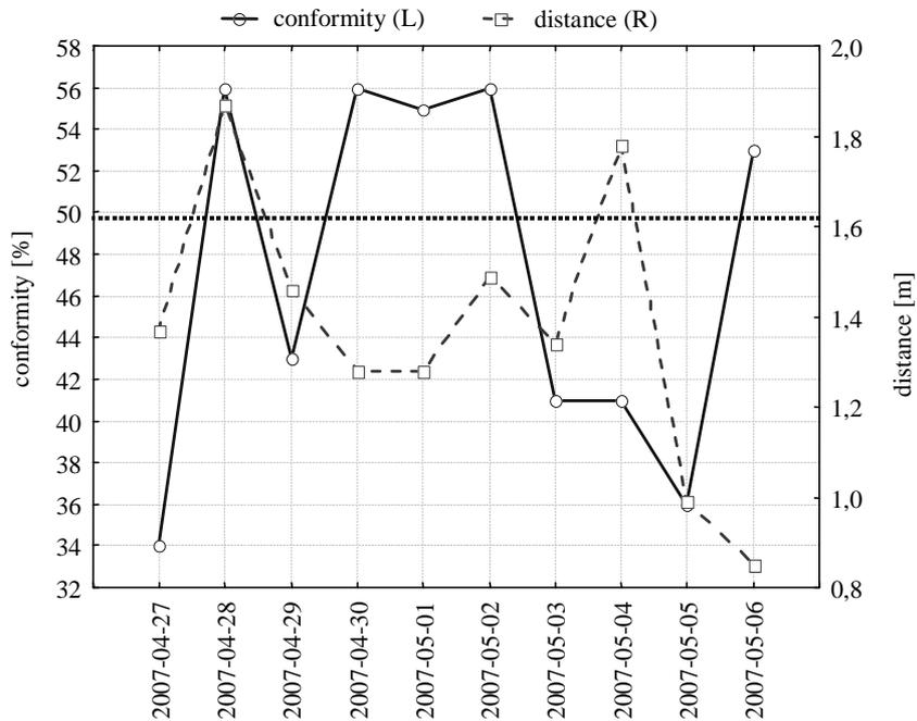
Fig. 1. Distance between mean positions of antennas (dashed line) for each measuring session. Conformity of the satellite segment tracked by both receivers (firm line), real distance between antennas (dotted line)
