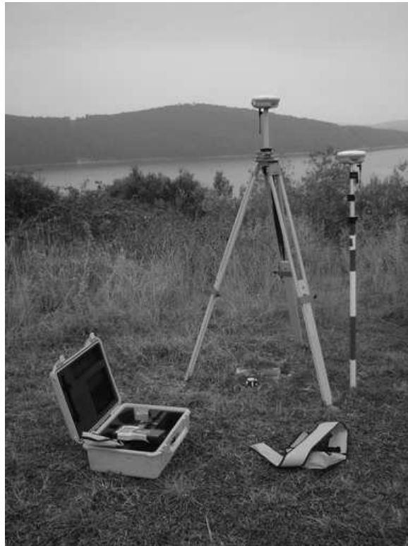
Figure 2. Measuring equipment: GPS/RTK base station
