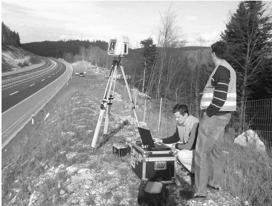
Fig. 5. Field team of the Faculty of Geodesy with 3D laser scanner
