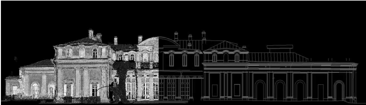
Fig. 7. From the point cloud to the 3D vector model – architectural heritage preservation
