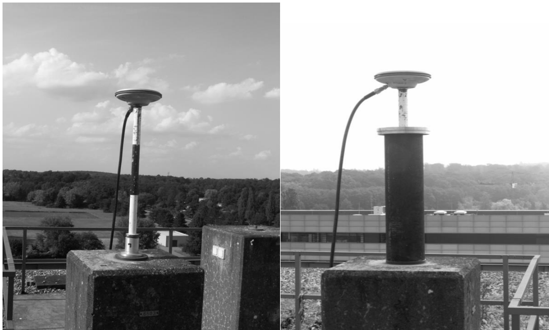
Fig. 5. Example of changing multipath environment in CEGRN sites: a reference configuration is shown on the left. A test configuration with a metallic disk underneath the antenna is shown on the right.
