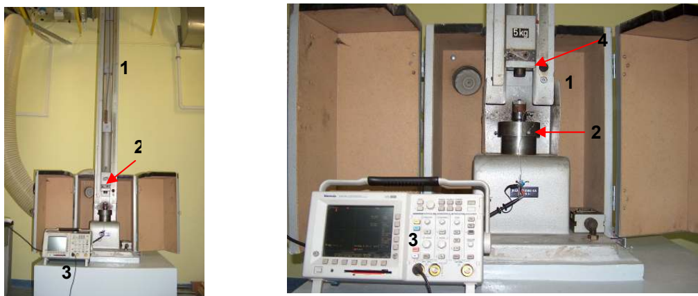
Fig. 1. The Caste hammer: 1 - the guide, 2 - the piezogenerator holder, 3 - the courses register, 4 - the weight
