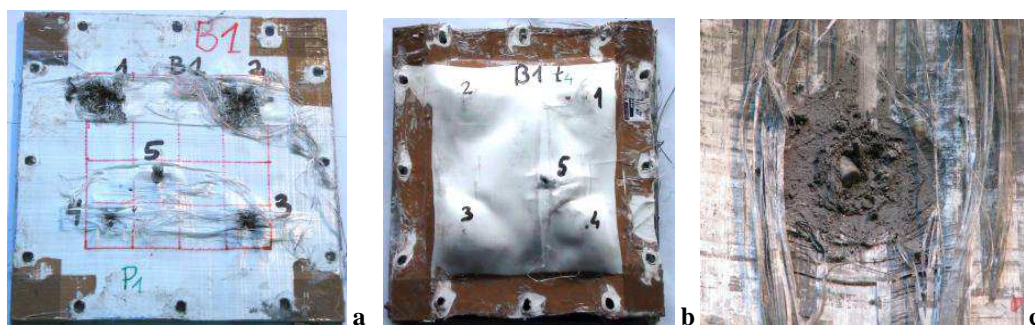
Fig. 7. Armour model of 350x350 mm with B 4 C ceramic (thickness - 19 mm, weight - 32 kg/m 2 ), (four projectiles stopped): front (a) and back (b) view after fivefold firing test and projectile remnants stuck inside the armour (c)
