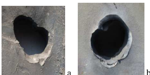
Fig. 10. The „witness” plate protected by the plate made from the steel subjected to the BT at 300°C (variant 2) after being fired: a – the front of the plate, b – the back of the plate
