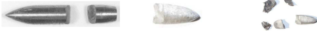
Fig. 12. The core of the 12.7 mm API projectile of the B-32 type after being fired at different materials
