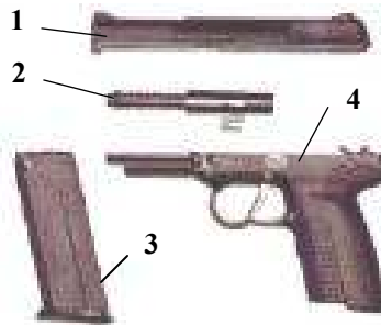
Fig. 6. The Five-seveN pistol partly separated: 1 - bolt, 2 - barrel, 3 - magazine, 4 - frame
