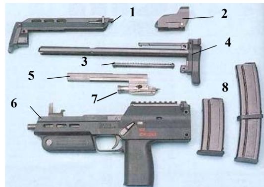
Fig. 4. The MP-7 submachine gun (partly separated) with the calibre of 4.6 mm: 1 - cover, 2 - collimator sight, 3 - recoil spring and guide, 4 - folding stock, 5 - lock frame, 6 - receiver, 7 - bolt, 8 - magazines
