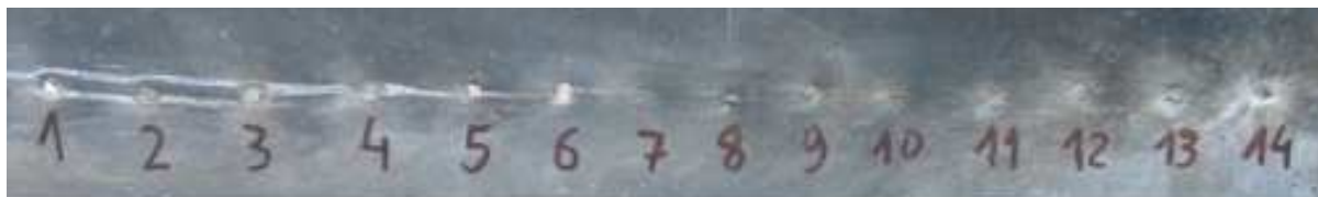
Figure 5. Mark on the RHA after firing B-32 12,7 mm bullets at all ceramic plates from ISiC (no. 1÷4, 7÷14) and ITME (no. 5÷6)
