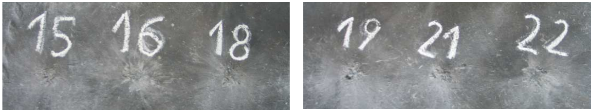
Figure 6. Marks on the RHA after firing at one-layered, large-sized Al_2O_3 ceramic plates from ISiC using 12,7 mm B-32 type bullets: no. 15÷22
