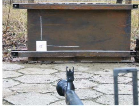
Figure 4. Stand using 12,7 mm machine gun, rotating stand with an armor plate and ceramic plate before firing
