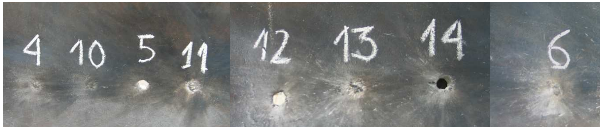
Figure 7. Marks on the RHA after firing at small-sized Al_2O_3 ceramic plates from ISiC, using 12,7 mm B-32 type bullets: no. 4÷6 (one-layered) and no. 12÷14 (double-layered)
