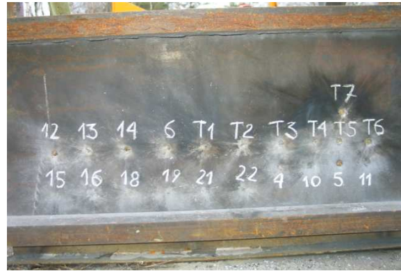
Figure 10. Marks on the RHA after firing at all ceramic plates from ISiC and ITME using 12,7 mm B-32 type bullets, - no. T1÷T4 (one-layered), b – no. T5÷T7 (double-layered)
