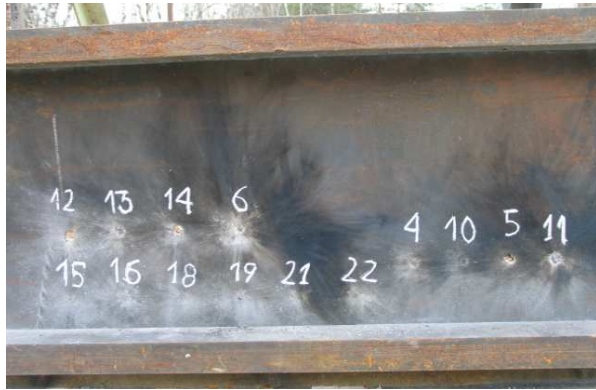
Figure 9. Marks on the RHA after firing at Al 2 O 3 ceramic plates from ISiC using 12,7 mm B-32 type bullets
