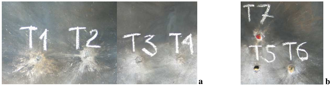
Figure 8. Marks on the RHA after firing at small-sized ceramic plates from ITME using 12,7 mm B-32 type bullets: a – no. T1÷T4 (one-layered), b – no. T5÷T7 (double-layered)
