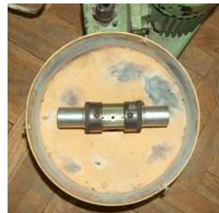
Fig. 3. Inserting of fuse to grip in whirling arm. Fig. 4. Pair fuses placed in whirling arm.
