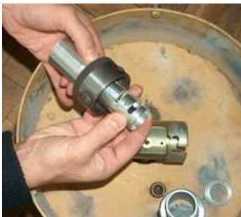
Fig. 3. Inserting of fuse to grip in whirling arm. Fig. 4. Pair fuses placed in whirling arm.
