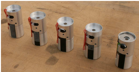
Fig. 5. Fuses without pyrotechnic and piezoelectric elements prepared for testing [5].
