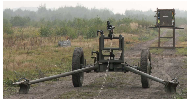
Fig. 11. View of stand for dynamic nondestructive testing of fuses.
