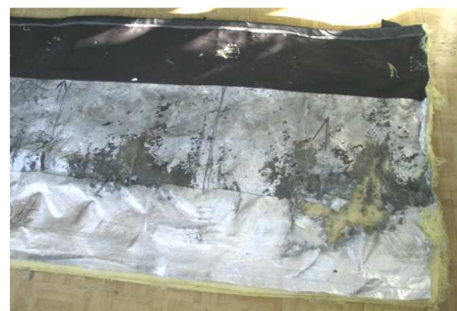
Fig. 13. A view to sample of destructed surface of cylinder cover version II
