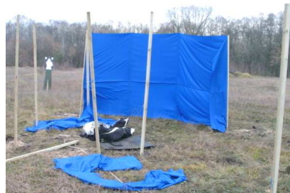
Fig. 12. A view to destruction of cylinder fibrous cover version II and screens after the explosion: a – cylinder cover; b – fabric screens
