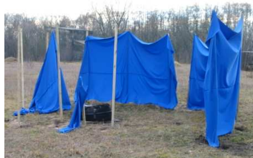
Fig. 18. Post-explosion view to: a – cylinder fibrous cover version III; b – fabric screens
