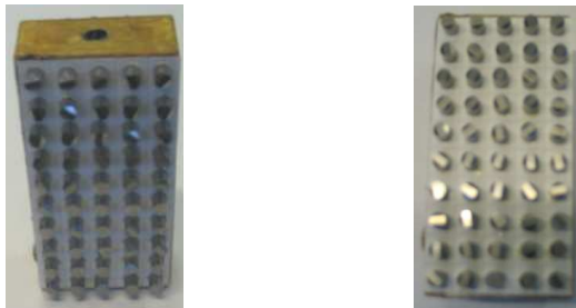
Fig. 2. TNT slab with bearing balls on its sides: a - Ø2 - 100x25 mm - 100 pcs, b - Ø3 - 100x25 mm - 100 pcs, c - Ø4 - 100x50 mm - 100 pcs, d - Ø5 - 100x50 mm - 100pcs
