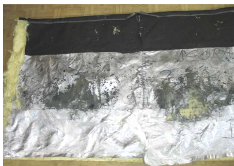
Fig. 13. A view to sample of destructed surface of cylinder cover version II
