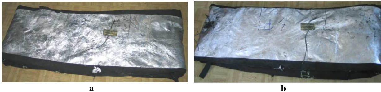
Fig. 21. View to inner side of cylinder where the (a) 3 mm and (b) 4 mm bearing balls operated
