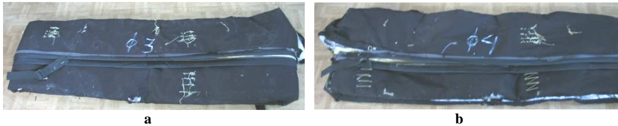
Fig. 20. View to outer side of cylinder where the (a) 3 mm and (b) 4 mm bearing balls operated
