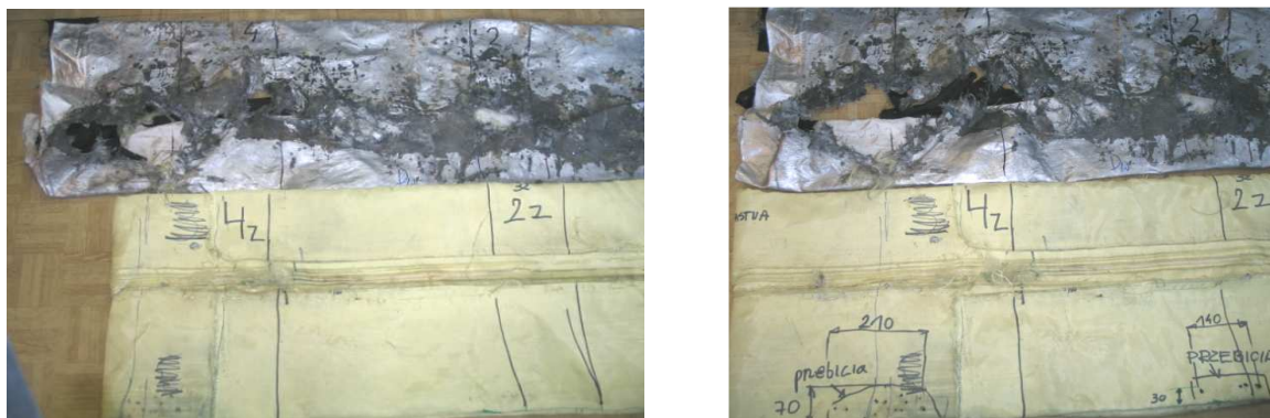
Fig. 9. A view to sample of destructed surface of cylinder fibrous cover version I
