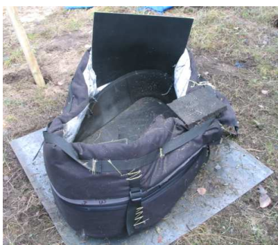
Fig. 18. Post-explosion view to: a – cylinder fibrous cover version III; b – fabric screens
