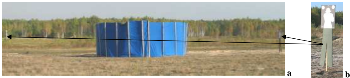
Fig. 6. The view of fabric screens (a) surrounding the cylinder cover with the TNT and fragments before explosion and the shields – soldier silhouettes (b) located ~ 10 m away from the explosion centre
