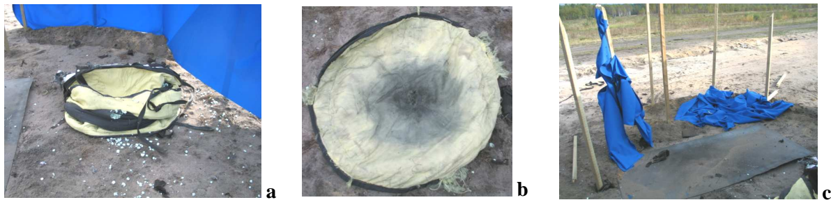
Fig. 8. A view to destruction of cylinder fibrous cover version I and the screens after the explosion: a – cylinder cover; b – cover lid; c – fabric screens
