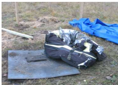
Fig. 12. A view to destruction of cylinder fibrous cover version II and screens after the explosion: a – cylinder cover; b – fabric screens
