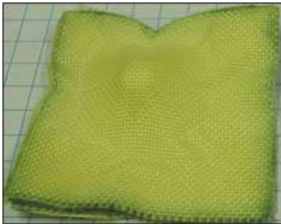
Fig. 3. Kevlar fabric with shear thickening fluid, after impact by a fragment simulating projectile
