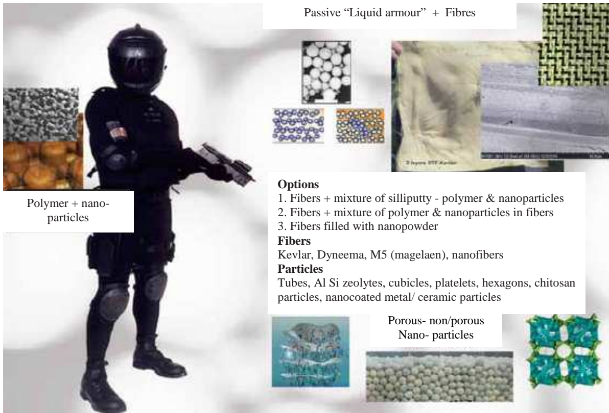
Fig. 2. Anti-ballistic materials for suit
