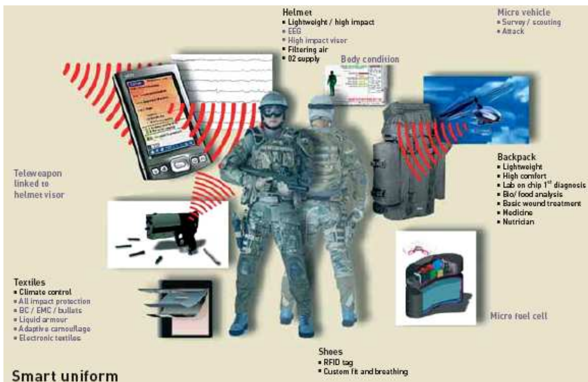
Fig. 10. Smart uniform with the different type of sensors
