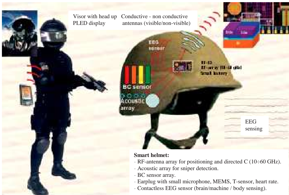
Fig. 12. Smart helmet with antenna sensor array (ASA)
