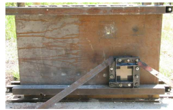
Fig. 5. Model of composite armour without a frame (a) and in a frame (b) on the RHA plate before firing with 14,5 mm B-32 type armour-piercing bullets
