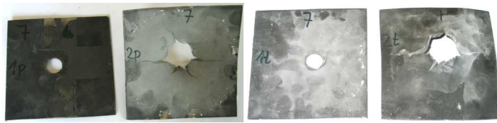
Fig. 12. Elements of composite armour's model 7 after firing with B-32 14,5 mm bullet
