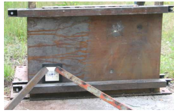
Fig. 5. Model of composite armour without a frame (a) and in a frame (b) on the RHA plate before firing with 14,5 mm B-32 type armour-piercing bullets
