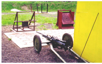
Fig. 4. Stand using 14,5 mm machine gun, rotating stand with an armour plate and ceramic plate before firing
