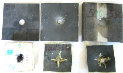
Fig. 10. Elements of composite armour's model 5 after firing with B-32 14,5 mm bullet
