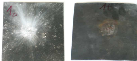
Fig. 6. Elements of composite armour's model 1 after firing with B-32 14,5 mm bullet
