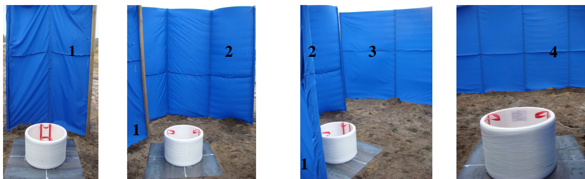
Fig. 11. View of cylindrically shaped fabric shields at various distances of 1÷4 m (marking 1÷4) with the "Episafe" attenuator and TNT bar with fragments before the explosion
