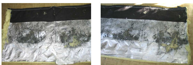
Fig. 14 View of demonstration damages to the surface of protection I cylinder
