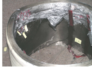
Fig. 23. View of the lower inside part of "Episafe" attenuator: (a) in a place for and near handle 1 - direction I and at the same time between handles 1 and 2 - direction II and (b) in a place for and near handle 2 - direction III and at the same time between handles 2 and 1 - direction IV
