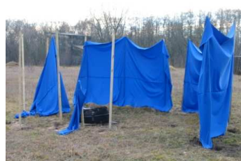
Fig. 17. View after explosion: a – fibrous protection version III; b – fabric shields
