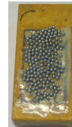
Fig. 8. A TNT bar with bearing balls stuck on two 100x50 mm walls; a - 200 balls Ø 4, b - 200 balls Ø 3 mm
