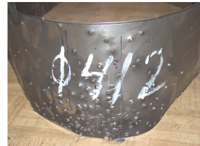
Fig. 18. View of the 2 nd sheet from the outside after an impact of fragments of 3 mm diameter (a) and 4 mm diameter (b)
