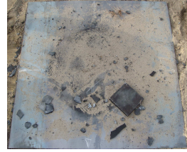
Fig. 22. View of sheets after detonation of the TNT bar with fragments in the "Episafe" attenuator, directly (a) and after cleaning sand off (b)
