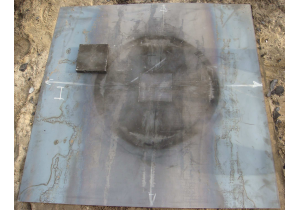
Fig. 22. View of sheets after detonation of the TNT bar with fragments in the "Episafe" attenuator, directly (a) and after cleaning sand off (b)
