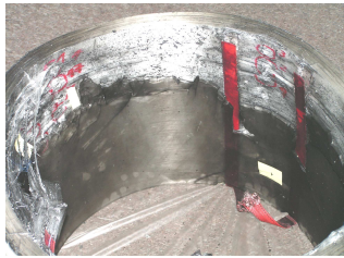
Fig. 21. View of "Episafe" attenuator and shields after detonation of the TNT bar with fragments
