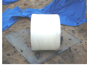
Fig. 21. View of "Episafe" attenuator and shields after detonation of the TNT bar with fragments
