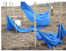
Fig. 21. View of "Episafe" attenuator and shields after detonation of the TNT bar with fragments
