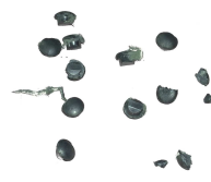
Fig. 15. View of damages to the shock absorbing layer of protection I (a) and deformed standard fragments
