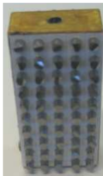
Fig. 7. A TNT bar with 100 standard fragments stuck on two 100x50 mm walls of the TNT bar
