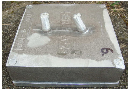
Fig. 8. Cassettes no. 1, 6 and 8 after the first drop on the concrete from the height of 12 meters
