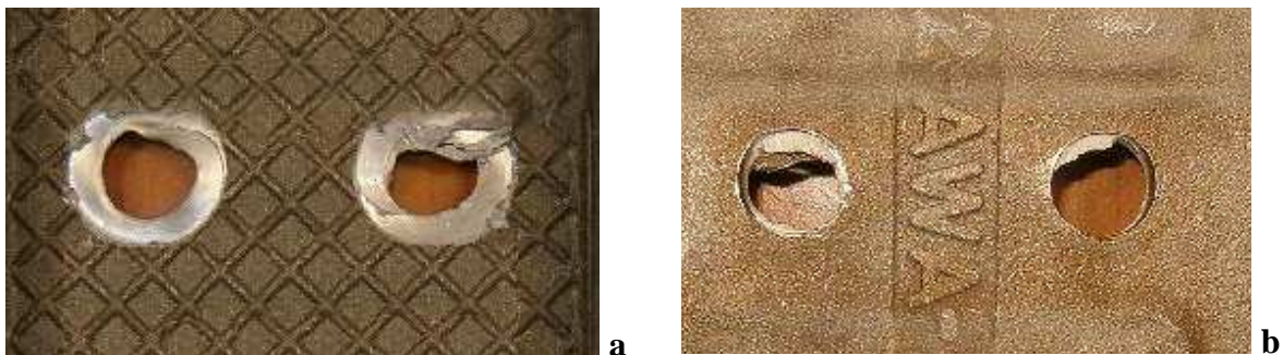
Fig. 3. The view of the cassette after the peel test of the screws: a – from the side of the tool, b – from the side of the screw [6]
