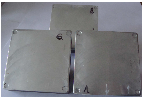
Fig. 8. Cassettes no. 1, 6 and 8 after the first drop on the concrete from the height of 12 meters
