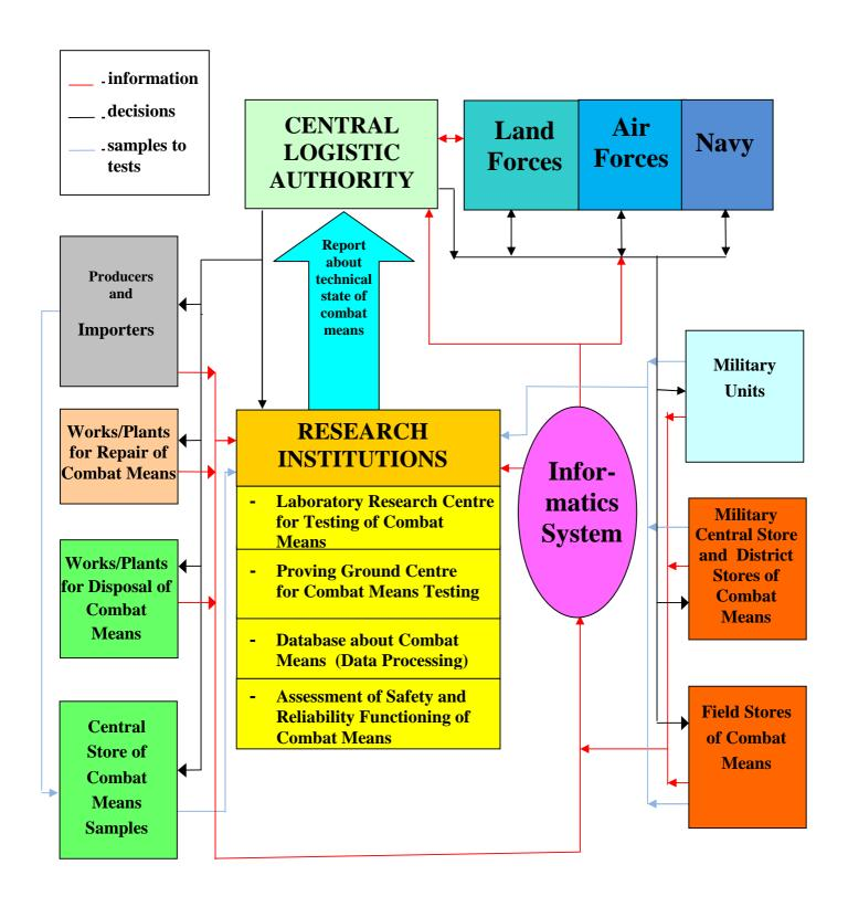
Figure 1. Servicing system of combat means including their quality and safety testing
