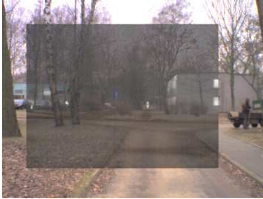
Fig. 3 The composite image obtained by fusion of visible camera image and thermovision camera image.
