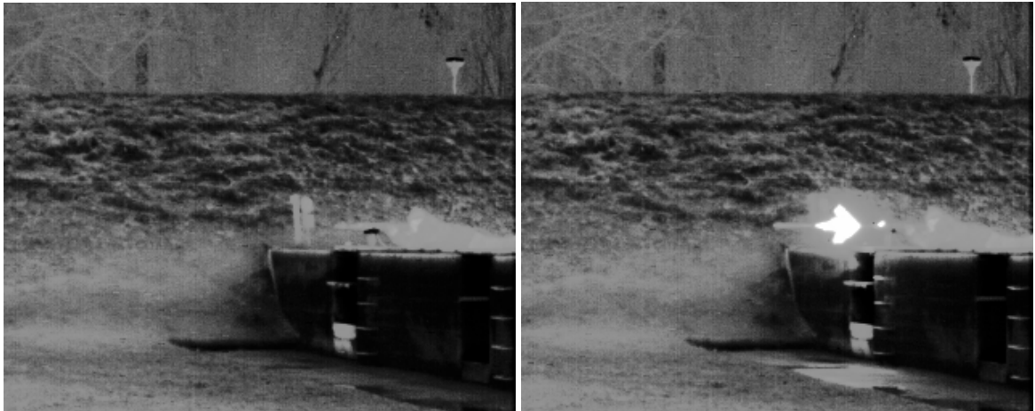
Fig. 3. Thermal signatures of sniper before and during shooting
