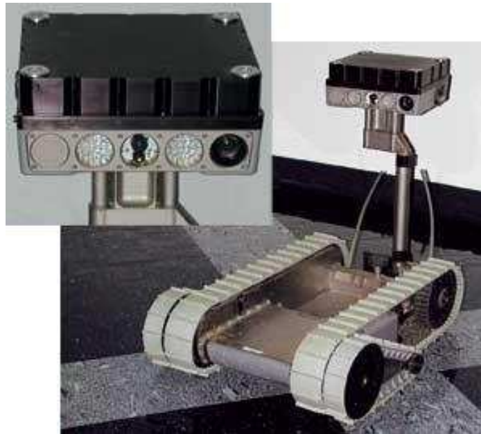
Fig. 3. REDOWL system mounted on PackBot tactical mobile robot.
