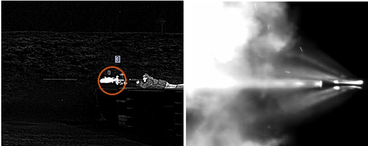
Fig. 1. Muzzle flash recorded in the 3-5 \mu\text{m} infrared range.
