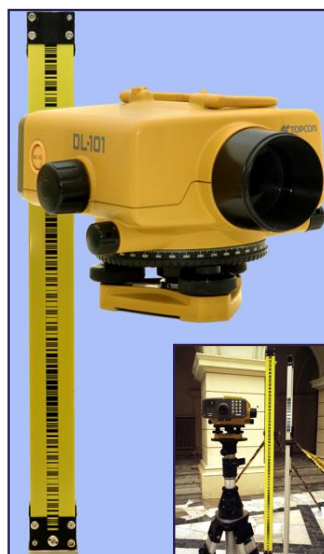
Fig. 2. A measuring set for precise levelling.
