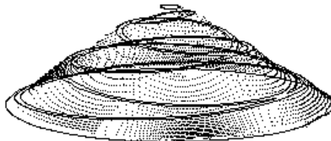
Fig. 8. Integration of scanning and polar method data; pathes edges are treated as break lines
