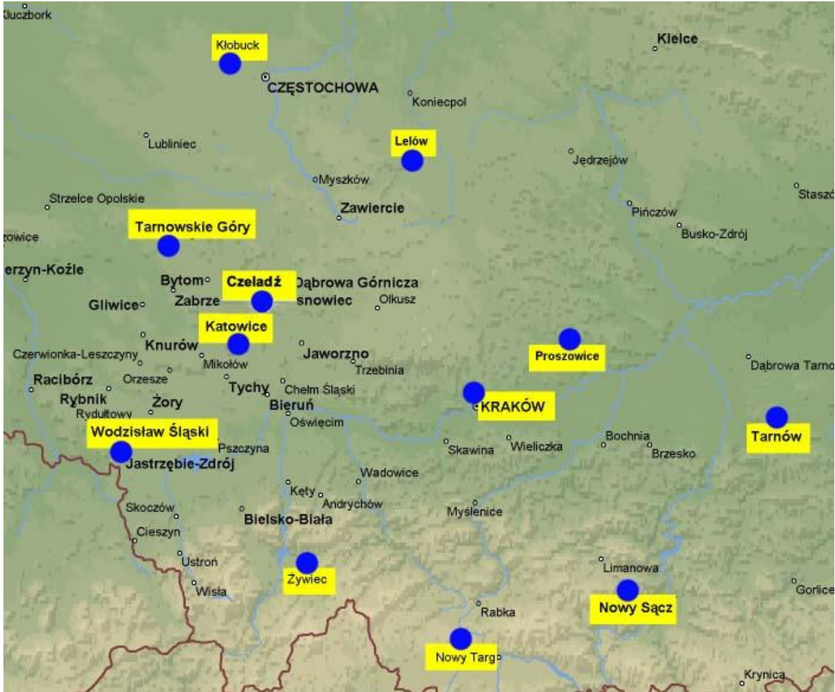
Fig. 1. Distribution of reference stations of Malopolski Satellite Positioning System [ www.gps.malopolska.pl ]
