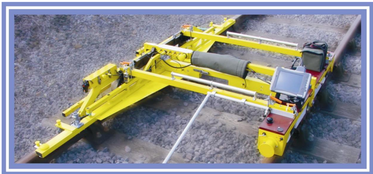
Fig.1. TQM (Track Quality Measurement) trolley.
