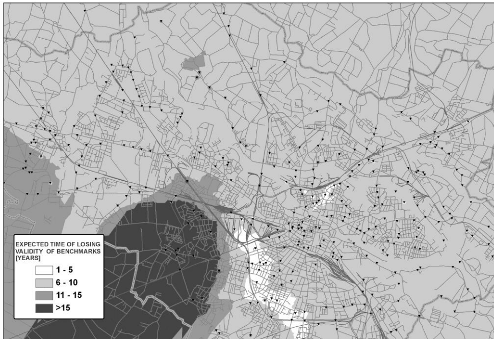
Fig. 6. Expected time of losing validity by benchmarks' ordinates since last measurement assuming rate of change calculated for the 1930 – 1998 time period.
