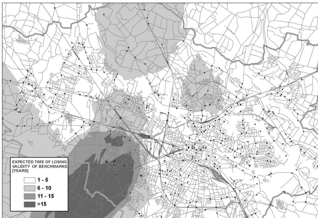
Fig. 8. Expected time of losing validity by benchmarks' ordinates since last measurement assuming rate of change calculated for the 1968 – 1998 time period.
