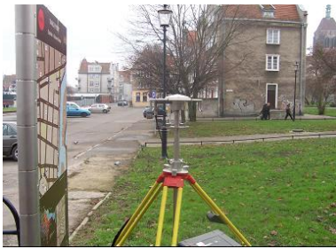
Fig.12. An obstacle (a metal information board) hampering GPS satellite signal reception at check point 6.
