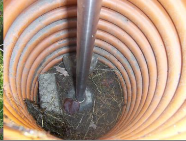
Fig. 8. Placing a pole on the benchmark. The benchmark is inside the sleeve situated at the pole end.
