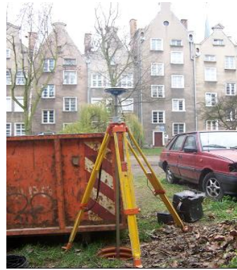
Fig.13. An obstacle (a steel container) hampering the correct positioning of the GPS aerial over check point 7.
