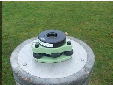
Fig. 5. Fastening and forced centring of the substage in the reference point mark head.
