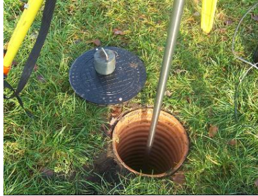
Fig. 7. Uncovered drain of the check point mark. The drain cover and the rubber shield of the benchmark visible on the side.
