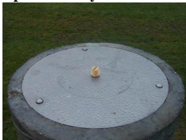
Fig. 4. The screw fastening substage in the reference point mark head.
