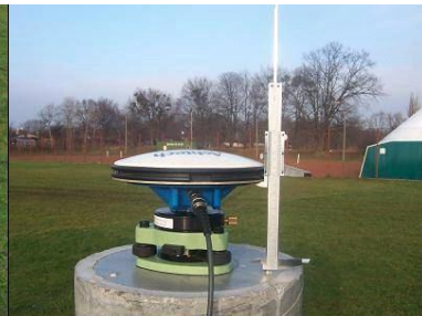
Fig. 6. Measurement of a GPS aerial altitude with a calliper in relation to one of the three reference points, situated on the reference mark head.
