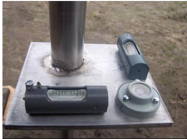
Fig. 10. A set of libels enabling the precise centring of the GPS aerial.
