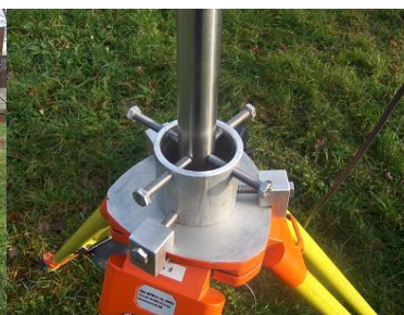
Fig. 3. Equipping a tripod with a pole-stabilising adjustable head.
