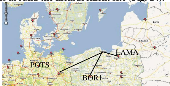
Rys.15. Connection of the reference points with the permanent stations of the IGS network: BOR1, LAMA, POTS.
