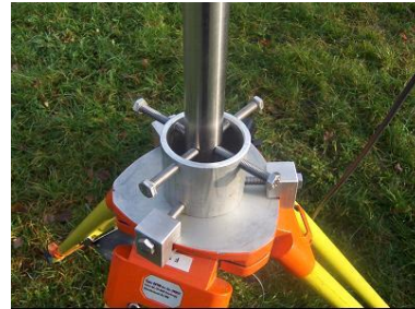
Fig. 11. An adjustable head, integrated with the tripod, enabling precisely vertical positioning of the pole (putting the bubbles of spirit levels at the upper position).
