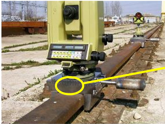
Fig. 5. Views of: a) rail stands in the process of examination and b) the detail of the body and the movable plate scales.
