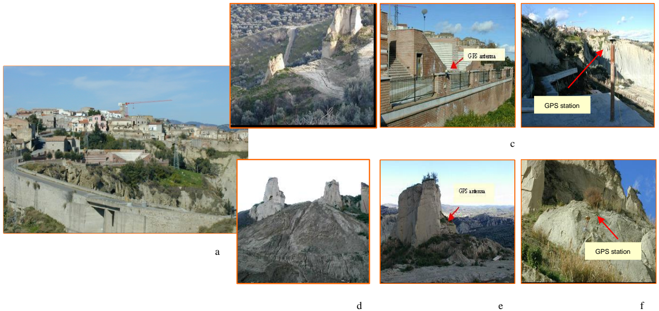
Fig. 8. Aliano landslide: evidence of the landslide displacement (a,b,d) and arrangement of GPS monitoring network
