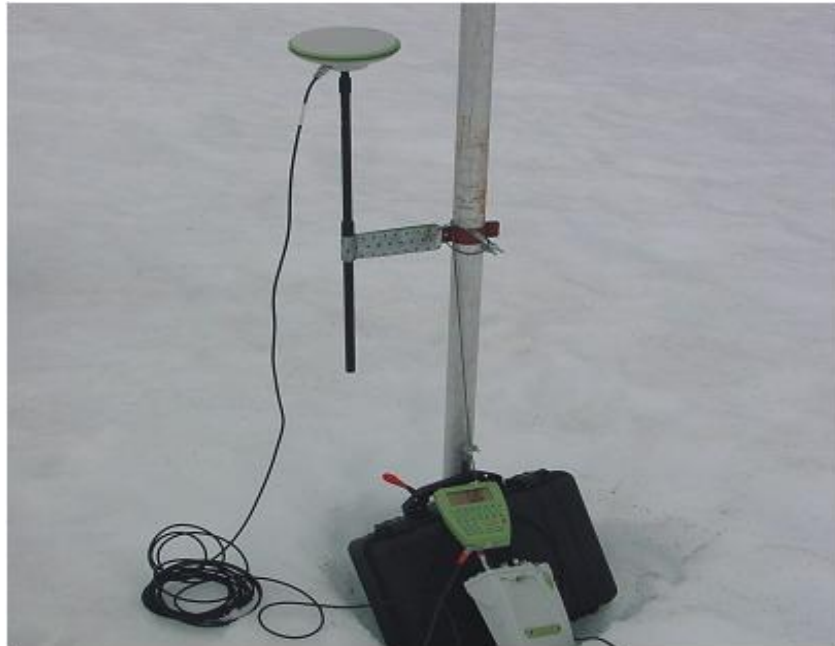
Fig. 3. Ablation pole with GPS antenna (A.Adamek)
