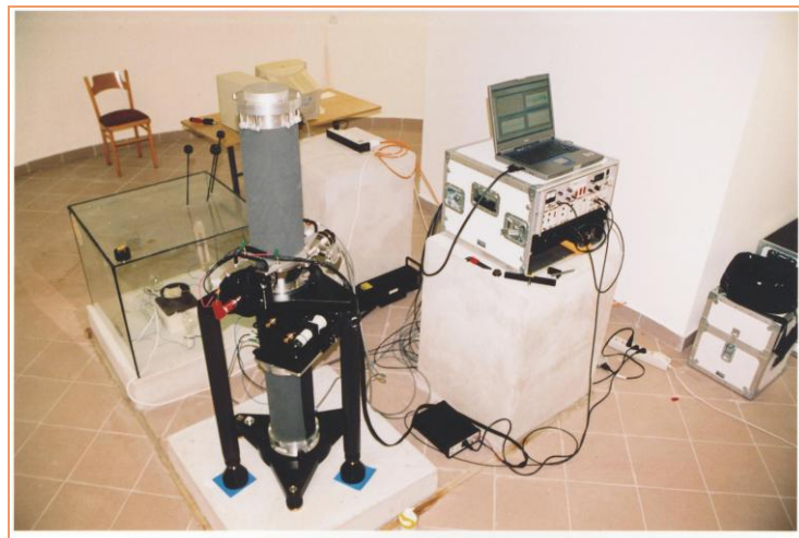
Fig. 5. FG5 No 230 gravity meter on station in Józefosław
